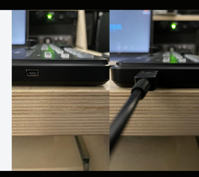
Plug the other end of the mini USB cable into black USB-C adapter. This should cause a white light to turn on and remain lit on the nanoKONTROL2.
